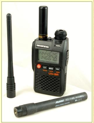
external antenna. The supplied antenna works well enough for me to use VHF and UHF repeaters 14 miles away with full signal strength on the functional S-meter.
