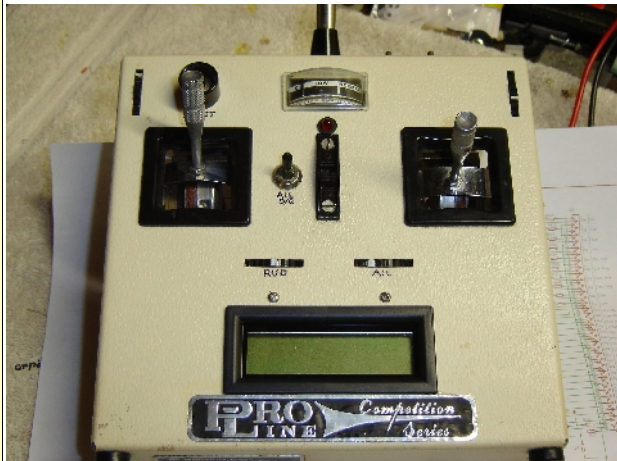
This is the front of the transmitter. The two control sticks steer the rudder, flaps, ailerons and elevator. The meter at the top displays RF output. The LCD display monitors battery voltage, control mixing values and a flight timer that counts up or down.
