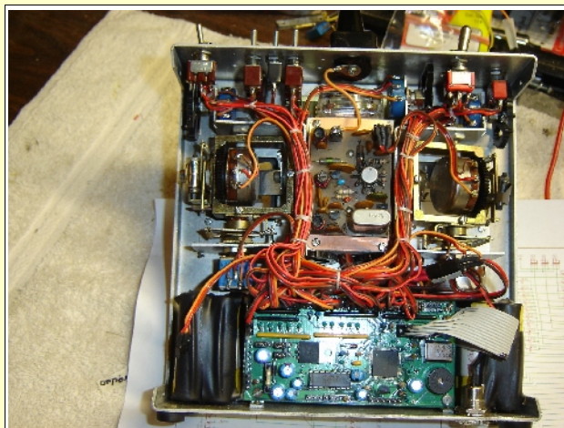
This is the rear of an RC transmitter. The circuit board at the bottom is the encoder while the RF circuit is just above. The various switches at the top control the flaps, spoilers and control mixing.
