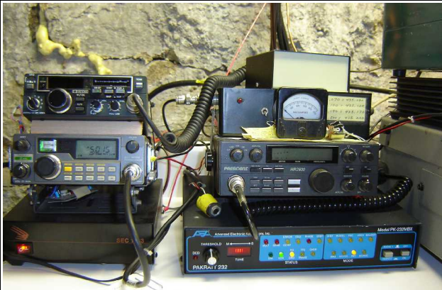
The modem is back in the stack on the bench. It connects to the computer via a serial cable. The Yaesu FT-290R all-mode two-meter transceiver is next to it and above the 20-amp switching power supply. The Yaesu is the RF link in FM.
