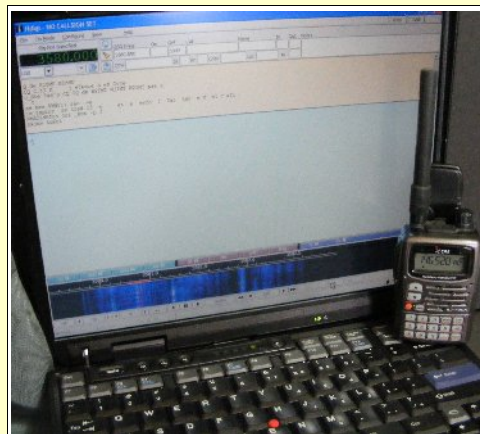
A fully functional NBEMS station with the minimum equipment necessary. (WA3UFN Photo)
